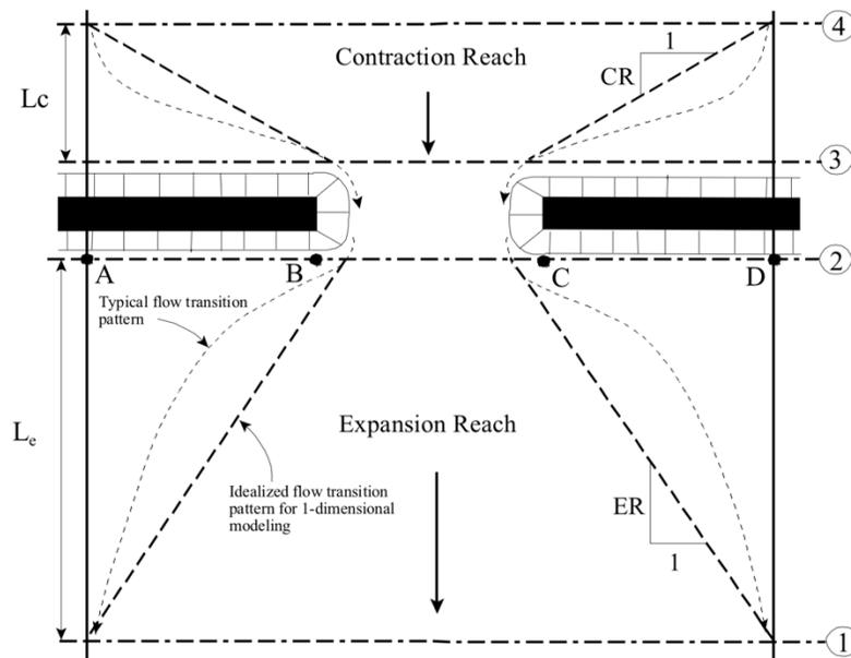
Figure 5-1 Cross Section Locations at a Bridge
